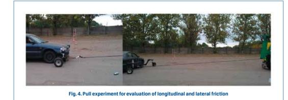
of the friction coefficient in the longitudinal direction of the vehicle is higher by 1.8–3.6 %. This trend is not in conflict with the properties described in the works reviewed by foreign scientists. So, using a skidcar system enables adjusting the friction characteristics equivalent to driving on wet or snowy road surface.
