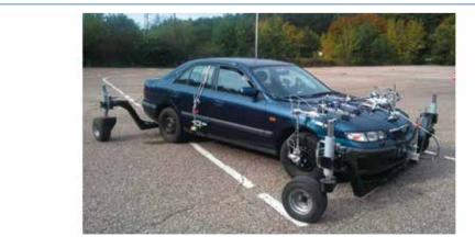
Fig. 5. Vehicle equipped with skidcar system and dynamic parameters measure sensors
