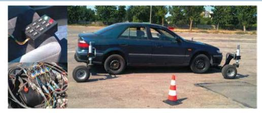
Fig. 1. Vehicle equipped with skidcar system and system control panel with 12V hydraulic power pack
